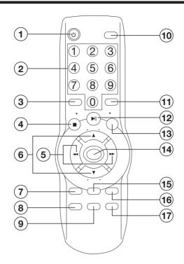
1. U POWER Press POWER to turn the unit ON or OFF
